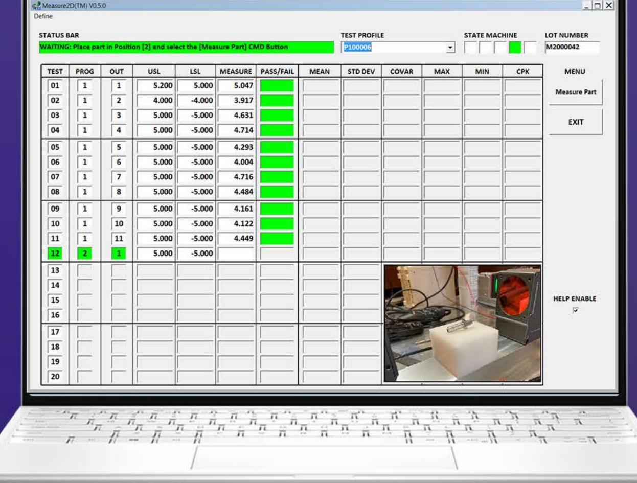
• Run Time: Automatic direct exporting/saving of measurement data to Microsoft Excel in "Ready to Print" Format == xlsx format. The Software has the capability of exporting over 1,000,000 data measurements directly to Microsoft Excel which far exceeds the Keyence TM-H1 limit of 65,535.
